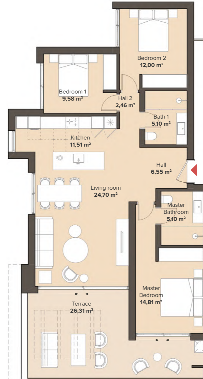
FIRST FLOOR APARTMENT
